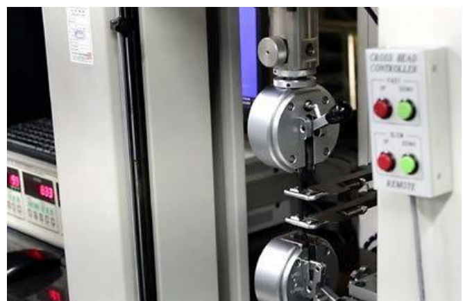
Mechanical test for tensile strength and elongation
