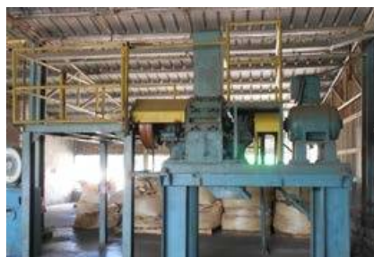
The PVC Granulator Machine granulates stripped and bled-out PVCs.
