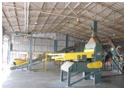
The Eldan Recycling Machine that separates copper from plastic
