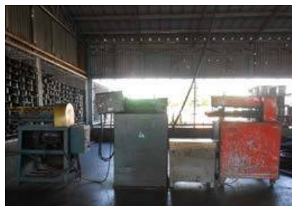
The Stripping Machine that recovers copper from scrap big insulated cables
