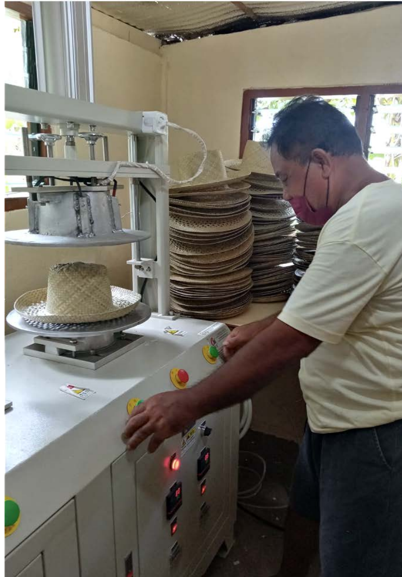
Through the use a hat-blocking machine, the quality of weavers' products is improved.
