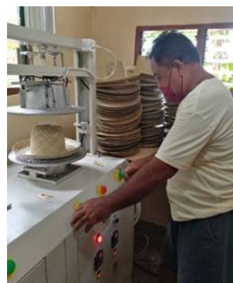
With a hat-blocking machine, the quality of weavers' products is improved.
