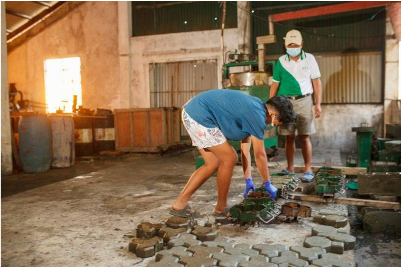
The War on Plastic project is successfully gaining traction in engaging the communities to reduce the use of single-use plastic and segregate it. Once segregated, the plastic is cook with used cooking oil through the extrusion process using a densifier machine. The resulting products are hardened tiles that can be used in schools and community's playgrounds.
